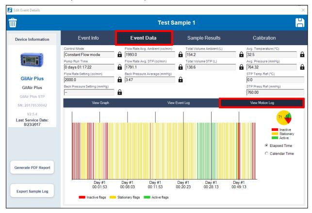
The bar graph shows the type of motion that the pump recorded at the time. The proportions of each of the 3 types of recorded motion are displayed in the pie chart and are the same numbers that are reported on the pump's event review screen. The user motion type is broken down into ACTIVE motion (walking), STATIONARY motion (wearing, but not walking), and INACTIVE motion (not wearing).
